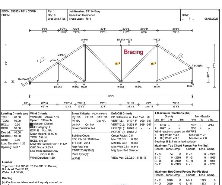
(a) Continuous lateral restraint equally spaced on member.
