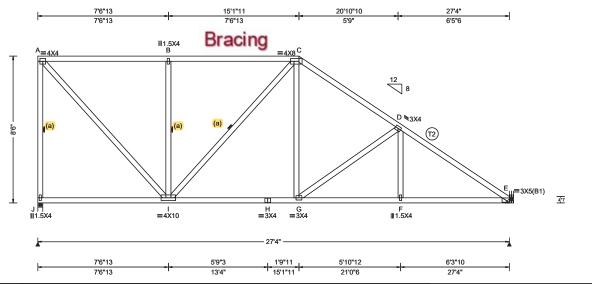
Loading Criteria (psf) TCLL: 20.00 TCDL: 10.00 BCLL: 0.00 BCDL: 10.00 Des Ld: 40.00 NCBCLL: 10.00 Soffit: 2.00 Load Duration: 1.25 Spacing: 24.0 "
