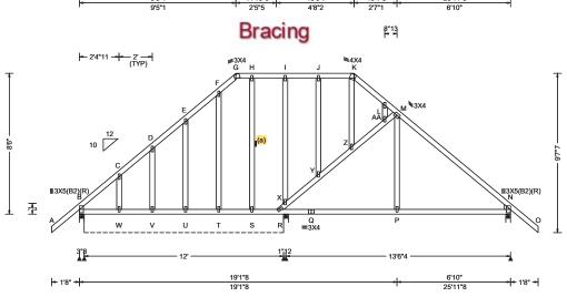
Loading Criteria (psf) TCLL: 20.00 TCDL: 10.00 BCLL: 0.00 BCDL: 10.00 Des Ld: 40.00 NCBCLL: 10.00 Soffit: 2.00 Load Duration: 1.25 Spacing: 24.0 "
