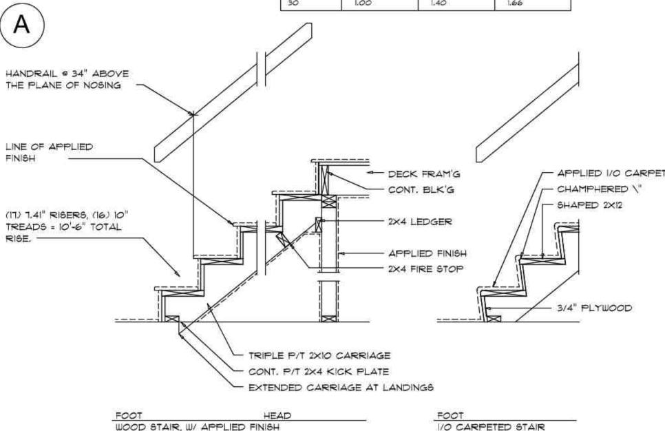
Typical Stair DETAIL SCALE: 3/4" = 1'-0"
