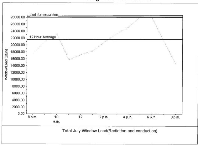
Warning: This application has glass areas that produce relatively large heat gains for part of the day. Variable air volume devices may be required to overcome spikes in solar gain for one or more rooms. A zoned system may be required or some rooms may require zone control.
