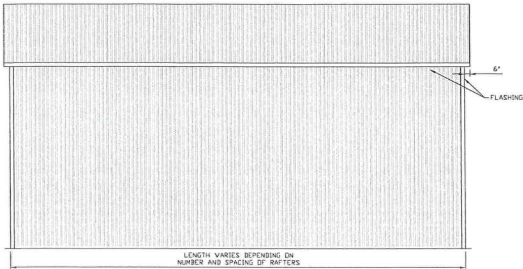
TYPICAL SIDE ELEVATION VERTICAL ROOF/SIDING SCALE: 1/8" = 1'-0"
