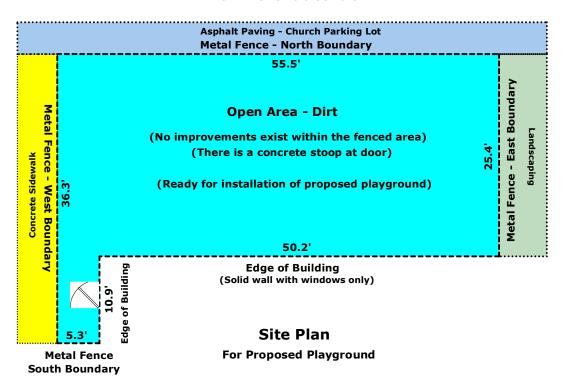
NOTE: The site dimensions represent the area located within the interior of the metal fence and the edge of building.
