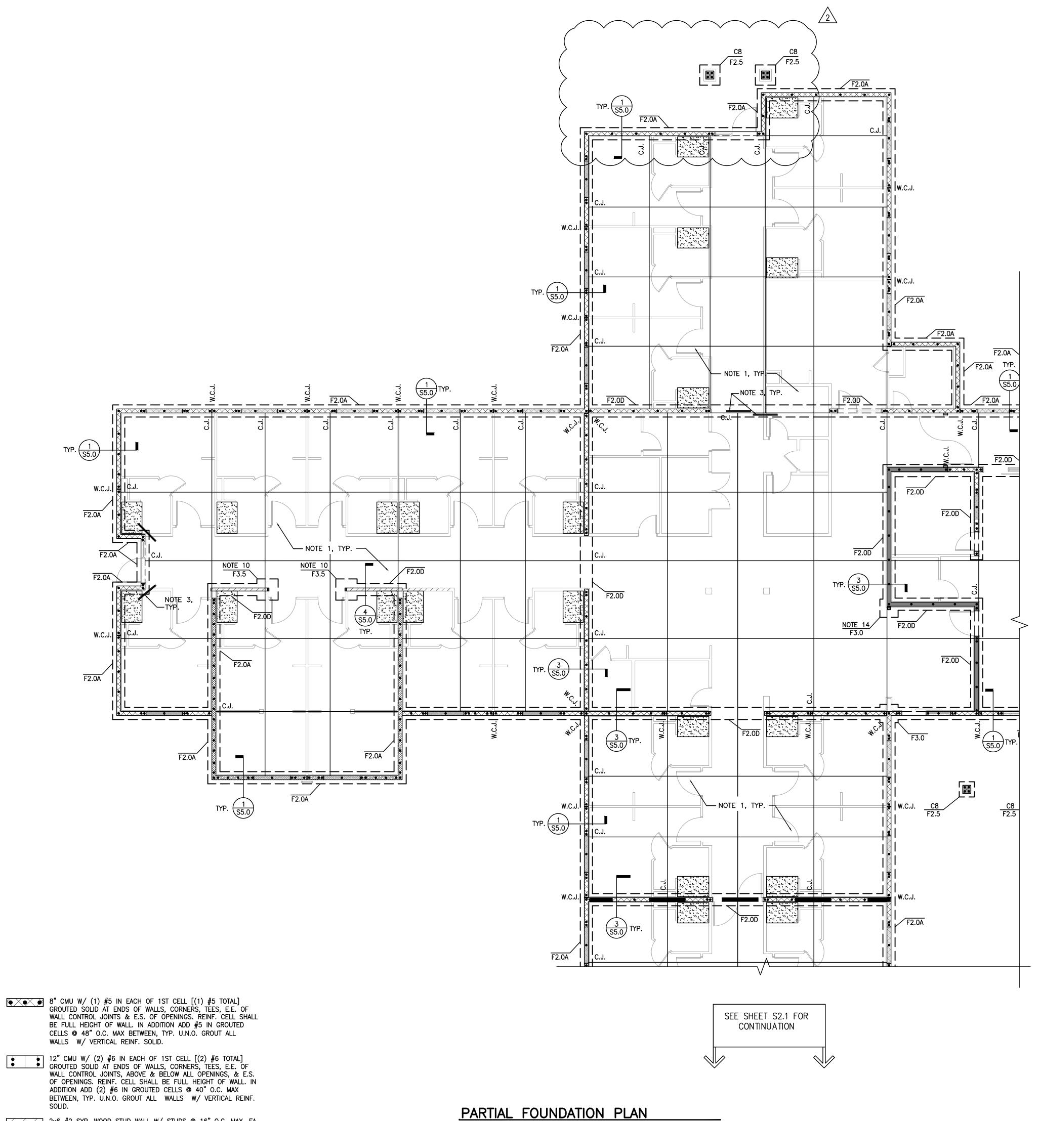
OF OPENINGS, REINF. CELL SHALL BE FULL HEIGHT OF WALL. IN ADDITION ADD (2) #6 IN GROUTED CELLS @ 40" O.C. MAX BETWEEN, TYP. U.N.O. GROUT ALL WALLS W/ VERTICAL REINF.
