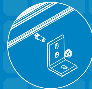
INTEGRATED BONDING MICROINVERTER MOUNT w/ WIRE MANAGEMENT
