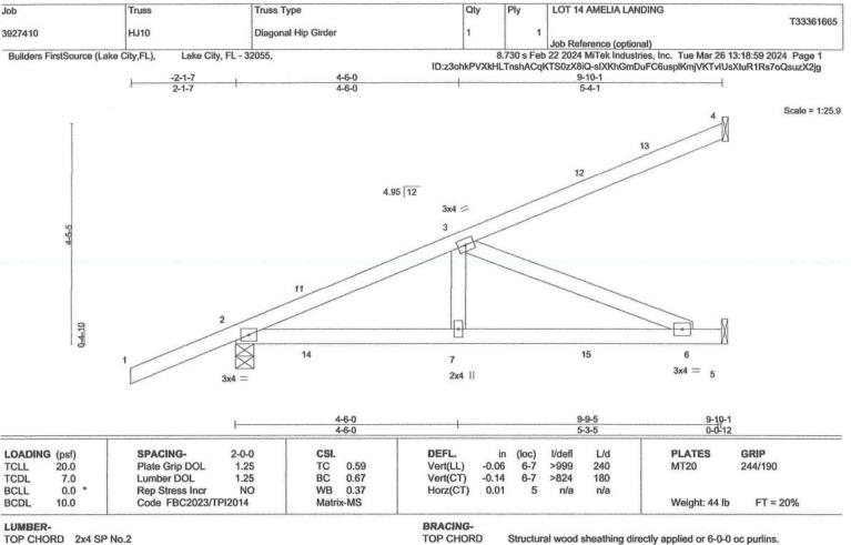
Rigid ceiling directly applied or 9-11-9 oc bracing.
