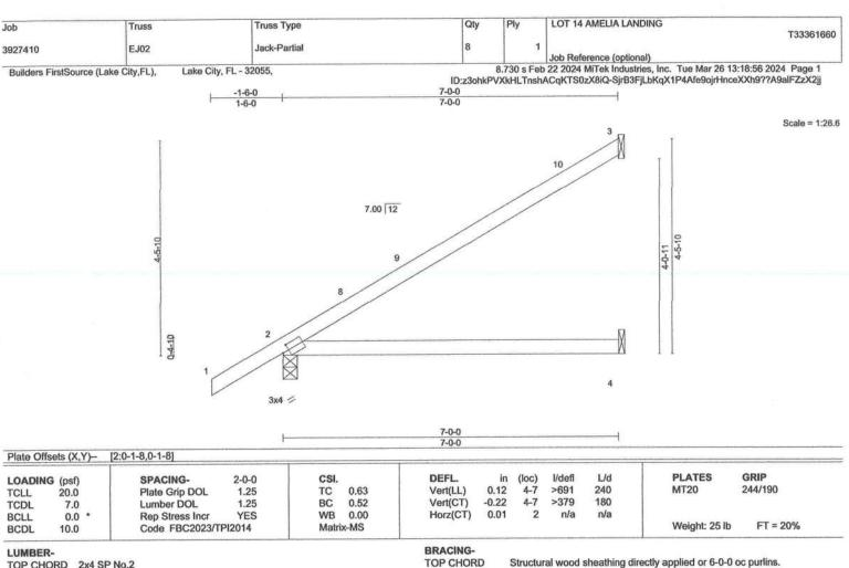
Rigid ceiling directly applied or 10-0-0 oc bracing.
