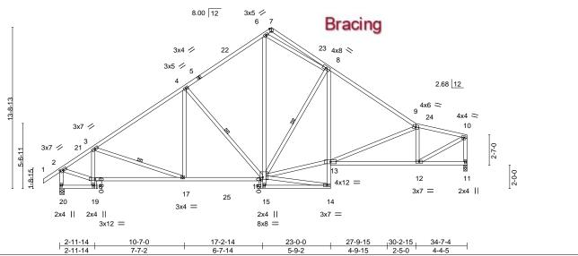
Plate Offsets (X,Y)--[2:0-3-3,0-1-8], [7:0-2-0, Edge], [16:0-2-8,0-2-4] LOADING (psf) SPACING-CSI. DEFL. (loc) I/defI L/d **TCLL** 20.0 Plate Grip DOL 1.25 TC 0.51 Vert(LL) -0.14 12-13 >999 360
