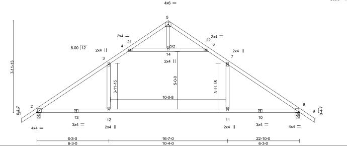
LOADING (psf) SPACING-CSI. DEFL. in (loc) I/defI L/d **PLATES** GRIP **TCLL** 20.0 Plate Grip DOL 1.25 TC 0.83 Vert(LL) -0.54 11-12 >507 360 MT20 244/190 TCDL Vert(CT) 10.0 Lumber DOL 1.25 BC 0.85 -0.99 11-12 >277 240 WB Horz(CT) **BCLL** 0.0 Rep Stress Incr YES 0.17 0.03 n/a n/a BCDL 10.0 Code FBC2020/TPI2014 Matrix-AS Wind(LL) -0.31 12-17 >894 240 Weight: 105 lb FT = 15%
