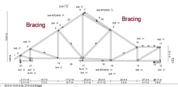
Plate Offsets (X,Y)--LOADING (psf) SPACING-CSI. DEFL. (loc) I/defI L/d **PLATES GRIP TCLL** 20.0 Plate Grip DOL 1.25 TC 0.68 Vert(LL) -0.18 18-19 >999 360 MT20 244/190 TCDL 10.0 Lumber DOL 1.25 BC 0.80 Vert(CT) -0.35 15-17 >999 240 MT20HS 187/143 WB **BCLL** 0.0 Rep Stress Incr YES 0.58 Horz(CT) 0.10 12 n/a n/a BCDL 10.0 Code FBC2020/TPI2014 Matrix-AS Wind(LL) 0.10 14-15 >999 240 Weight: 281 lb FT = 15%
