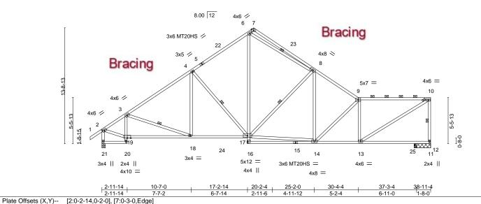
LOADING (psf) SPACING-CSI. DEFL. (loc) I/defl L/d **PLATES GRIP TCLL** 20.0 Plate Grip DOL 1.25 TC 0.73 Vert(LL) -0.18 14-16 >999 360 MT20 244/190 TCDL 10.0 Lumber DOL 1.25 BC 0.73 Vert(CT) -0.36 14-16 >999 240 MT20HS 187/143 WB **BCLL** 0.0 Rep Stress Incr YES 0.54 Horz(CT) 0.10 n/a n/a BCDL 10.0 Code FBC2020/TPI2014 Matrix-AS Wind(LL) 0.09 13-14 >999 240 Weight: 286 lb FT = 15%
