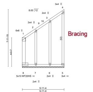
Plate Offsets (X,Y)--[5:Edge,0-1-8] LOADING (psf) SPACING-2-0-0 CSI. DEFL. (loc) I/defI L/d **PLATES GRIP TCLL** 20.0 Plate Grip DOL 1.25 ТС 0.89 Vert(LL) n/a n/a 999 MT20 244/190 TCDL вс MT20HS 10.0 Lumber DOL 1.25 0.82 Vert(CT) n/a n/a 999 187/143 WB **BCLL** 0.0 Rep Stress Incr YES 0.19 Horz(CT) 0.00 5 n/a n/a BCDL 10.0 Code FBC2020/TPI2014 Matrix-R Weight: 56 lb FT = 15%
