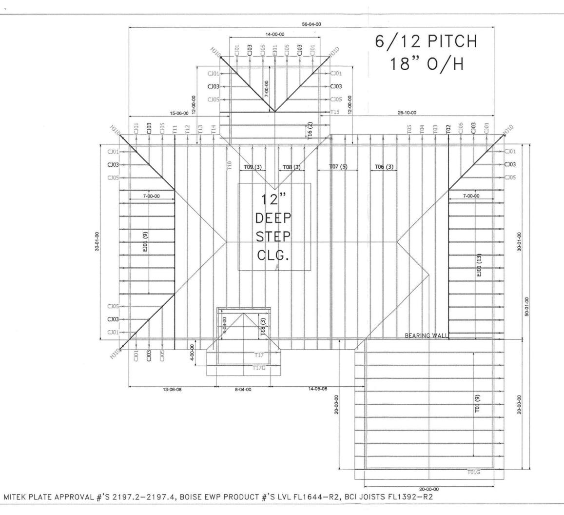
THE ARROW HEAD AT THE END OF THE TRUSS ON THE TRUSS PLACEMENT PLAN (LAYOUT) CORRESPONDS WITH THE LEFT SIDE OF THE INDIVIDUAL TRUSS DRAWING. USE THIS AS AN DRIENTATION GUIDE WHEN SETTING THE TRUSSES ON THE STRUCTURE.
