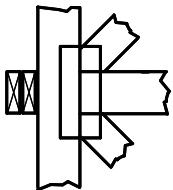
Indicates location where bearings (supports) occur. Icons vary but reaction section indicates joint number/letter where bearings occur. Min size shown is for crushing only.
