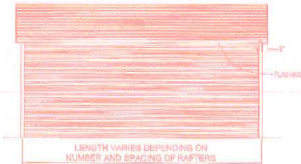
TYPICAL SIDE ELEVATION - HORIZONTAL ROOF SCALE: 1/8" = 1'
