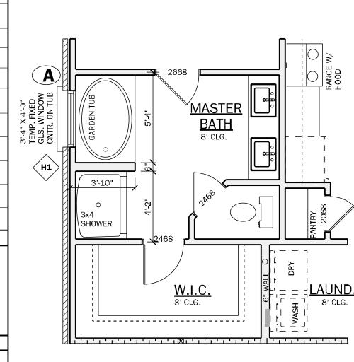
MASTER BA. OPTIONS 030 (1) PC. FIBERGLAS SHOWER IN LIEU OF LINEN CLOSET W/ (1) L.E.D. DISC LT. 3'-4" X 4'-0" TEMP. FIXED LS. WINDOW CNTR. ON TUB **OPTIONAL MASTER BATH**
