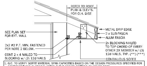
COMPONENT AND CLADDING LISTED IN THE DESIGN CRITERIA ON COVER PAGE. 2. 2x2 #2 MIN. P.T. W/ J-CHANNEL SECURED @ 24" O.C. FASTEN TO CMU W/ 3/16"x3" TITEN 2 @ 16" O.C (ALT. PAF 0.145/0.157 & 0.300 WASHER W/ MIN. 1" EMBEDMENT @ 16" O.C. IF WOOD WALL, DIRECT APPLY TO STRUCTURE W/ 0.148"x31/4" NAILS @ 16"0.0 . (F) CHANNEL APPLICATION: 2x2 NOT REQUIRED SEE (PA) INSTALLATION GUIDE
