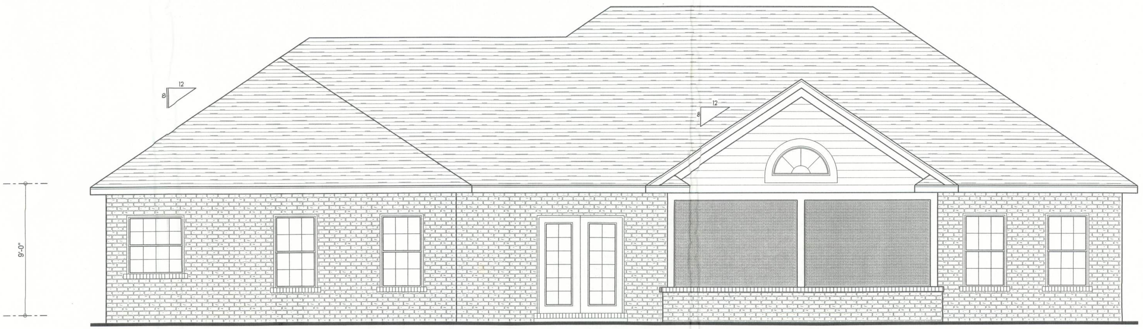
REAR ELEVATION SCALE: 1/4" = 1'-0"
