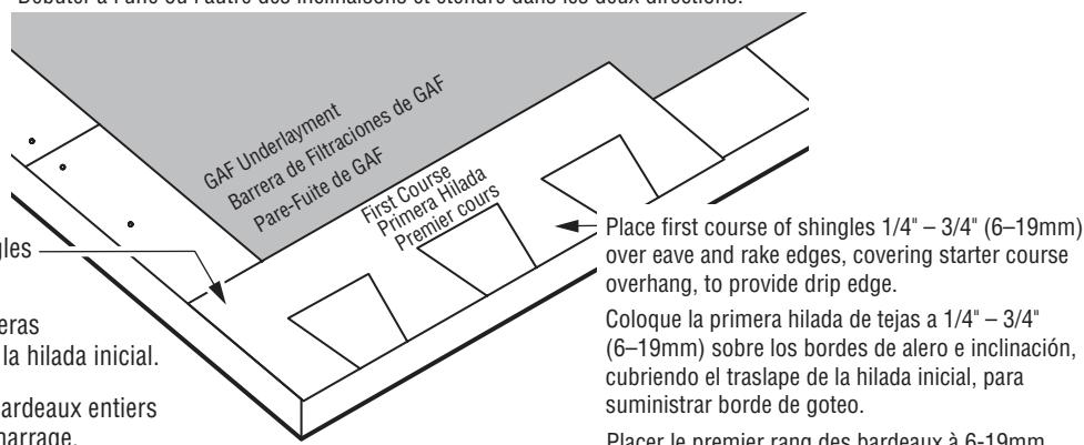
Place first course of shingles 1/4" – 3/4" (6–19mm) over eave and rake edges, covering starter course overhang, to provide drip edge.
