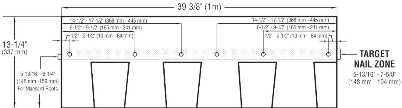
**ENHANCED NAILING PATTERN\*:** Nail shingles with 6 nails approximately 6 7/8" (174 mm) from bottom of shingle, in nailing area, as shown. Nails must not be exposed. For mansard roofs (21:12 and above), nail a nominal 6" (152 mm) from the bottom of the shingle and hand-seal shingles.
