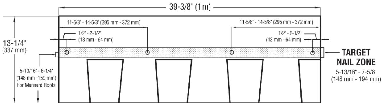
**STANDARD NAILING PATTERN:** Nail shingles with 4 nails approximately 6 7/8" (174 mm) from bottom of shingle, in nailing area, as shown. Nails must not be exposed. For mansard roofs (21:12 and above), nail a nominal 6" (152 mm) from the bottom of the shingle and hand-seal shingles.
