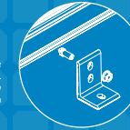
INTEGRATED BONDING MICROINVERTER MOUNT w/ WIRE MANAGEMENT
