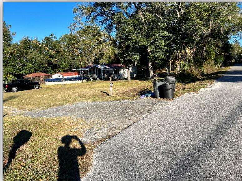
Per Columbia County LIDAR, the road elevations vary from 123.5' +/- to 123.7' +/- and the existing ground elevation is 116.5' +/- . The minimum finished floor elevation shall be 118.00'. The finished floor elevation of 118.00' is sufficient to protect the home from water damage in a base flood event.
