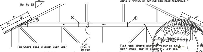
Note: If purlins or sheathing are not specified on the flat top of the base truss, purlins must be installed at 24' o.c. max. and use Detail A.
