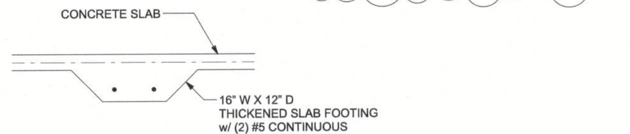
F2 S-2 INTERIOR BEARING FOOTING
