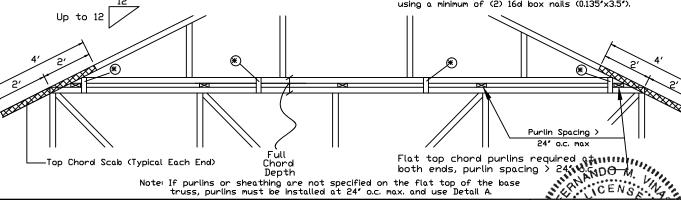
Note: If purlins or sheathing are not specified on the flat top of the base truss, purlins must be installed at 24" o.c. max. and use Detail A.
