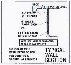
NOTE: IF ANY PART OF THE POOL **ENCROACHES UPON THE ANGLE OF** REPOSE, PLACE STEEL @ 6" o.c. EA WAY
