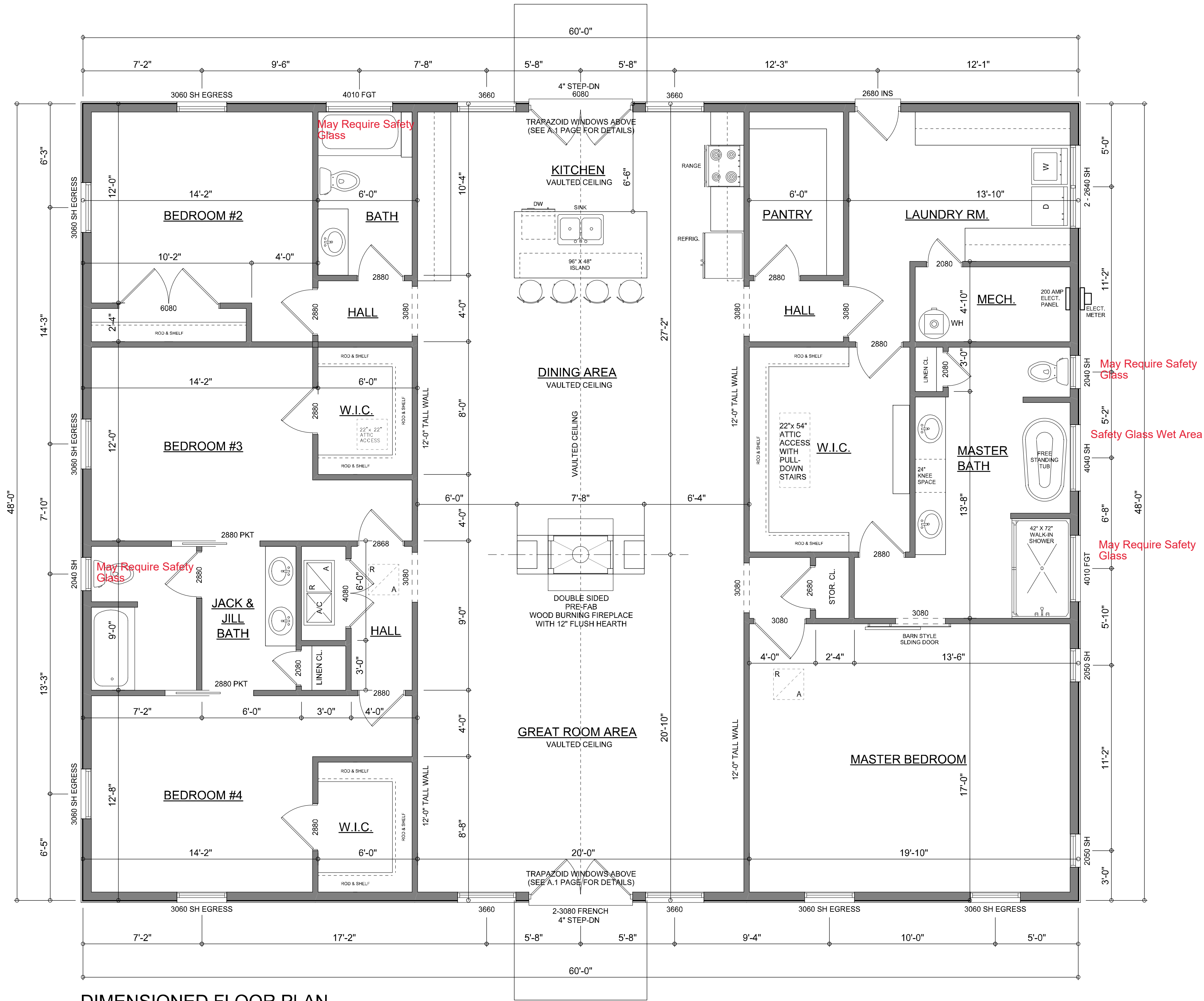
DIMENSIONED FLOOR PLAN SCALE: 1/4" = 1'-0" NOTE: ALL WALLS SHALL BE 10'-0" UNLESS OTHERWISE NOTED.
