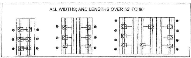
HOMES WITH 5/12 ROOF PITCH REQUIRE. PER FLORIDA REGULATIONS 6 systems for home lengths up to 52' and 8 systems for homes over 52' and up 80' One stabilizer plate and frame the required at each lateral bracing system
