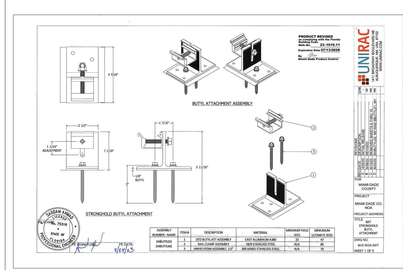
ATTACHMENT DETAIL FOR SHINGLE ROOF
