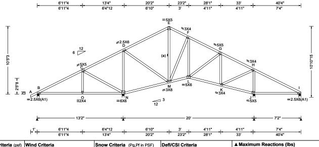
505 /295 /289 1582 /-/-/991 /33 /-/689 1109 /-/18 318 /-/192 /35 /-Wind reactions based on MWFRS Brg Wid = 4.0 Min Req = 1.5 Min Req = 1.9 Brg Wid = 4.0 Brg Wid = 4.0 Min Req = 1.5 Brg Wid = 4.0 Min Req = 1.5 Bearings B, N, J, & I are a rigid surface.
