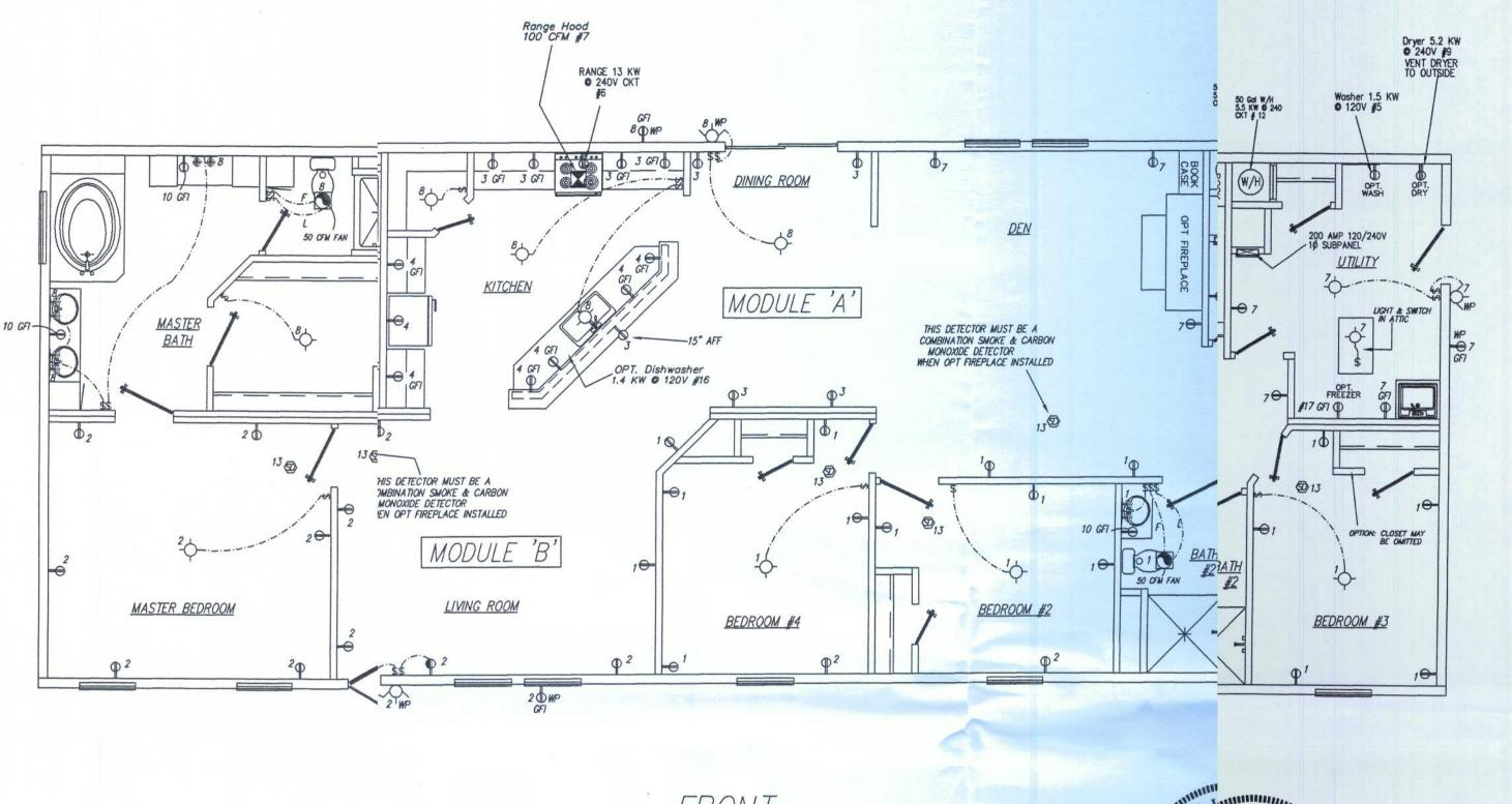
NOTE: ALL RECEPTACLES INSTALLED ON 15 AMP AND 20 AMP CIRCUITS MUST BE LISTED AS 'TAMPER RESISTANT'
