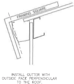
GUTTER INSTALLATION DETAIL (ONLY IF PROVIDED)
