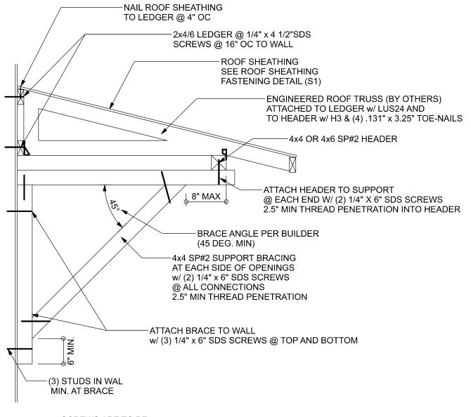
SCREWS ARE TO BE TOE-SCREWED OR ANGLED DO NOT SCREW INTO END GRAIN
