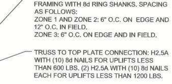
7/16" OSB ROOF DECK FASTENED TO
