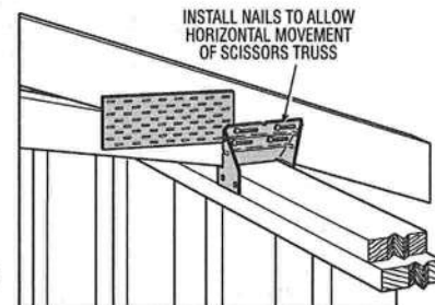
Typical TC24 Installation
