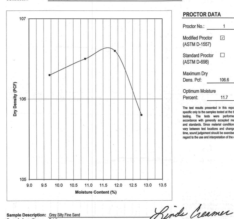
PROCTOR DATA 1 Proctor No.: 1 Modified Proctor (ASTM D-1557) Standard Proctor (ASTM D-698) Maximum Dry Dens. Pcf: 106.6 Optimum Moisture Percent: 11.7
