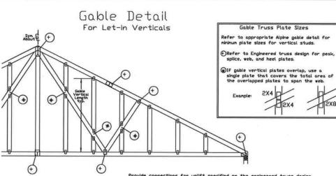
Provide connections for uplift specified on the engineered truss design. Attach each 'T' reinforcing member with
