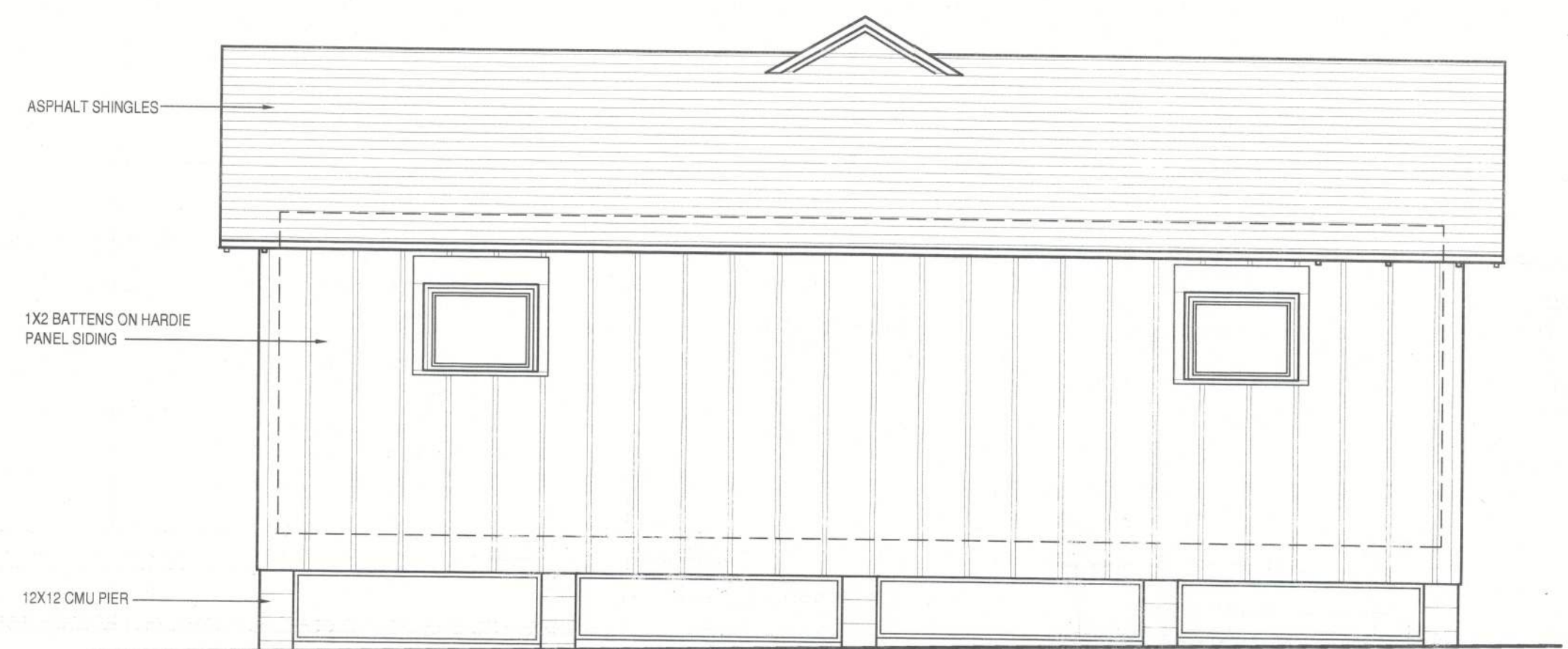
LEFT SIDE ELEVATION 1/4" = 1'-0"
