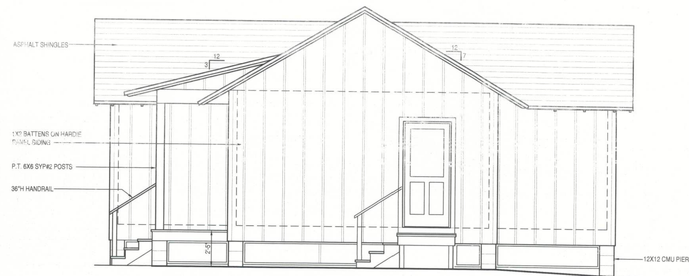
RIGHT SIDE ELEVATION 1/4" = 1'-0"
