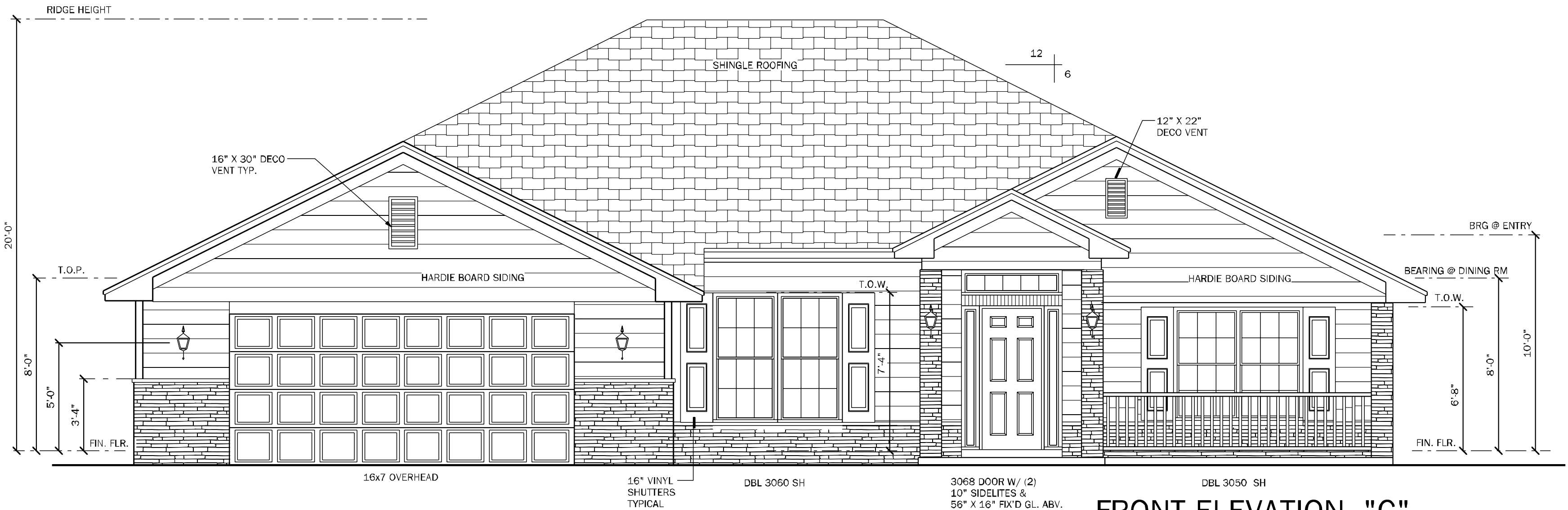
FRONT ELEVATION "C" SCALE: 1/4" =1'-0"
