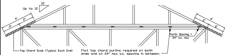
Piggyback cap truss slant nailed to all top chord purlin bracing with (2) 16d box nails (0.135"x3.5") and secure top chord with 2x4 #3 grade scab (1 side only at each end) attached with 2 rows of 10d box nails (0.128"x3") at 4" o.c.
