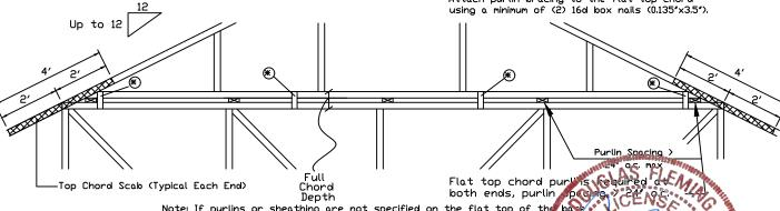
Note: If purlins or sheathing are not specified on the flat top of the base truss, purlins must be installed at 24" o.c. max. and use Detail
