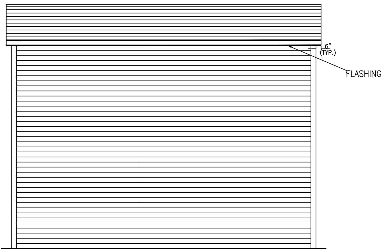
TYPICAL SIDE ELEVATION VERTICAL ROOF/SIDING SCALE: N.T.S.
