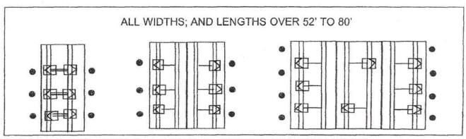
HOMES WITH 5/12 ROOF PITCH REQUIRE: PER FLORIDA REGULATIONS 6 systems for home lengths up to 52' and 8 systems for homes over 52' and up 80'. One stabilizer plate and frame tie required at each lateral bracing system.
