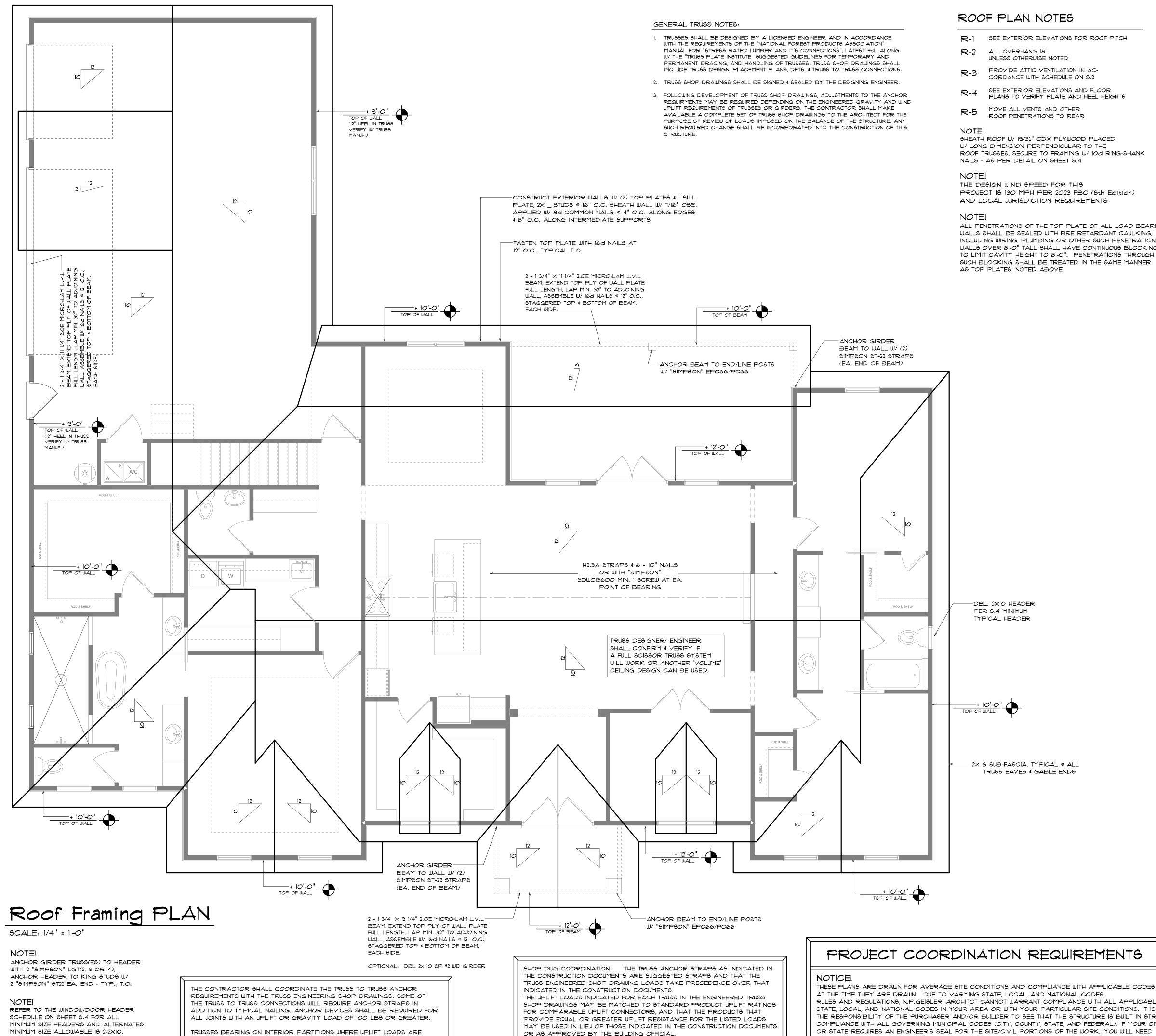
TRUSSES BEARING ON INTERIOR PARTITIONS WHERE UPLIFT LOADS ARE PRESENT SHALL REQUIRE ANCHORS OF EQUAL OR GREATER LOAD CAPACITY THAN THAT INDICATED BY THE TRUSS SHOP DRAWINGS, THE UPLIFT ANCHOR SYSTEM SHALL BE CONTINUOUS TO THE FOUNDATION.
