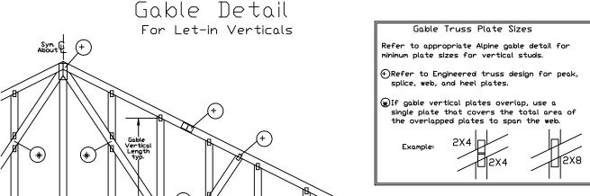
Provide connections for uplift specified on the engineered truss design.
