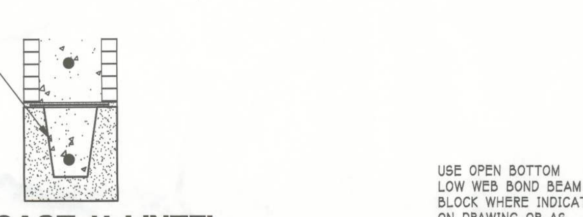
PRECAST U-LINTEL REINFORCEMENT AT OPENINGS SCALE: 1 1/2"=1'-0"
