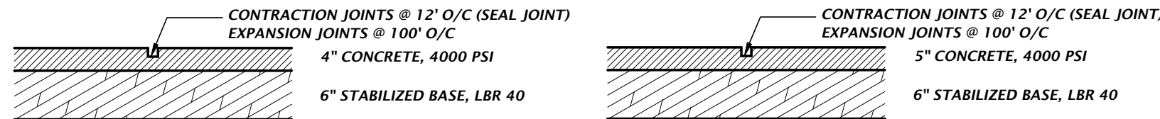
STANDARD DUTY CONCRETE DETAIL
