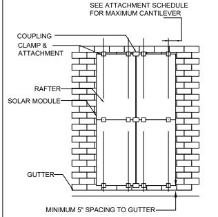
ECOFASTEN SOLAR ROCK-IT 4.0 MOUNTING DETAIL ECOFASTEN SOLAR ROCK-IT 4.0 RAIL-LESS MOUNTING SYSTEM INTEGRATED WITH FLASHING, COUPLINGS AND ADJUSTABLE CLAMP ATTACHMENTS
