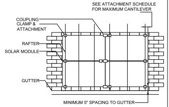
ECOFASTEN SOLAR ROCK-IT 4.0 MOUNTING DETAIL ECOFASTEN SOLAR ROCK-IT 4.0 RAIL-LESS MOUNTING SYSTEM INTEGRATED WITH FLASHING, COUPLINGS AND ADJUSTABLE CLAMP ATTACHMENTS
