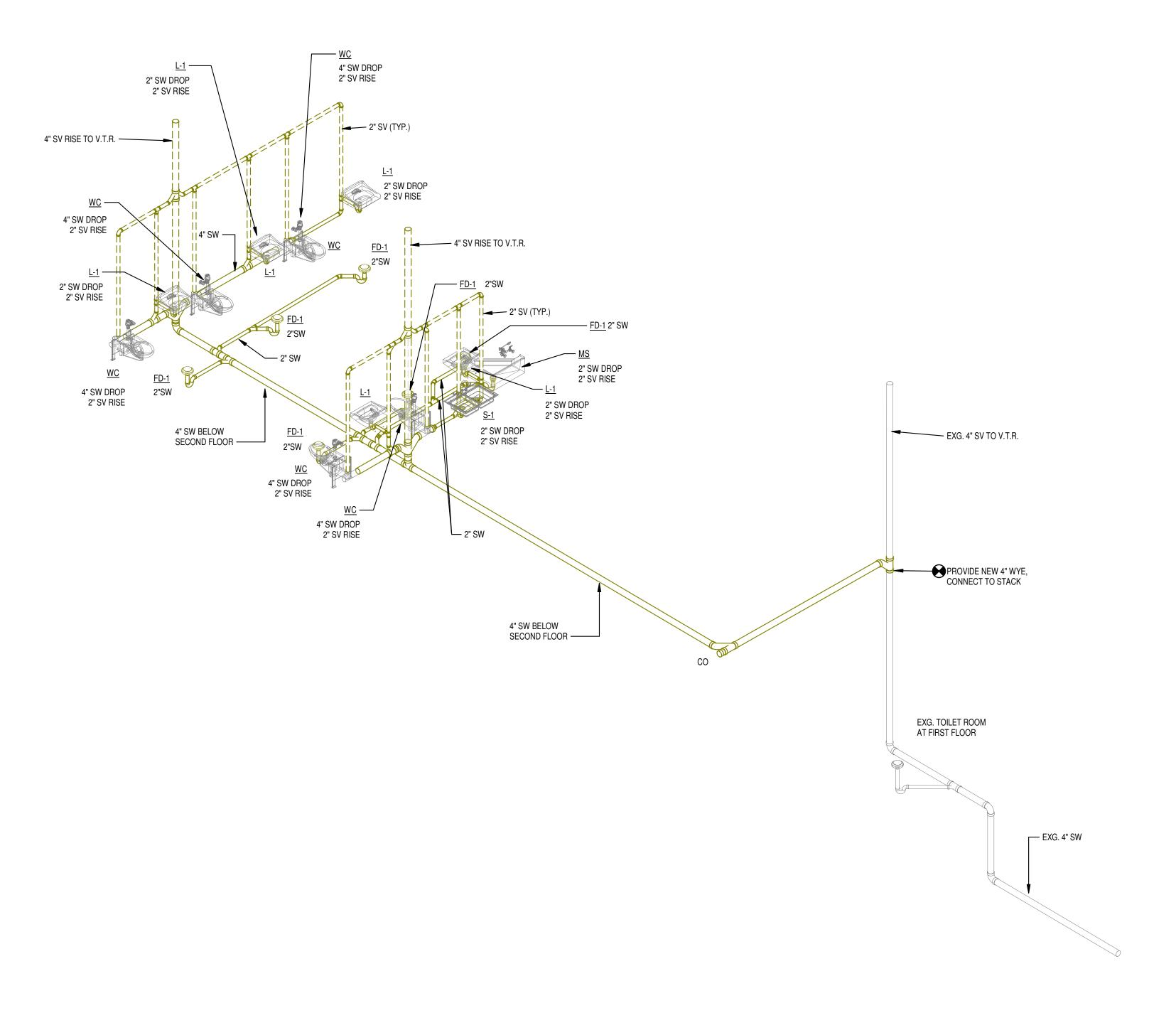
A3 DRAINAGE WASTE VENT RISER DIAGRAM - AREA 2 SCALE: NOT TO SCALE
