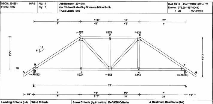
TCLL: 20.00 TCDL: 10.00 BCLL: 0.00 BCDL: 10.00 Des Ld: 40.00 **NCBCLL: 10.00** Soffit: 2.00 Load Duration: 1.25 Spacing: 24.0 \*
