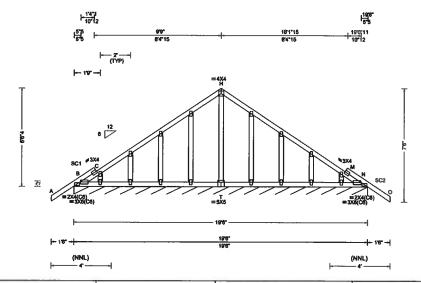
Loading Criteria (psf) TCLL: 20.00 TCDL: 10.00 BCLL: 0.00 BCDL: 10.00 Des Ld: 40.00 NCBCLL: 10.00 Soffit: 2.00 Load Duration: 1.25 Spacing: 24.0 \*
