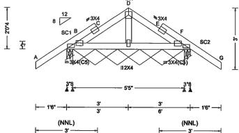
Loading Criteria (psf) TCLL: 20.00 TCDL: 10.00 BCLL: 0.00 BCDL: 10.00 Des Ld: 40.00 **NCBCLL: 10.00** Soffit: 2.00 Load Duration: 1.25 Spacing: 24.0 \*
