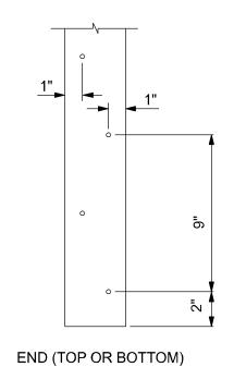
GIRDER COLUMN DETAIL SCALE: 1/2" = 1'-0"
