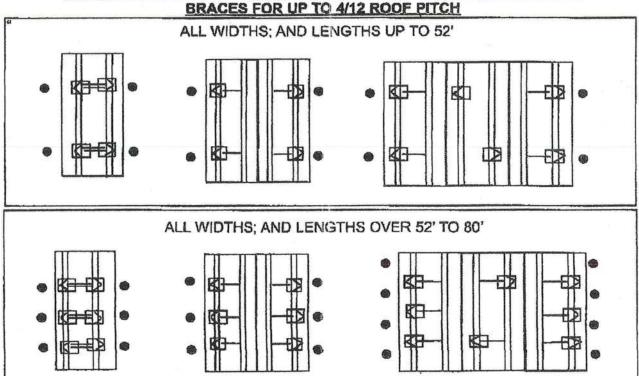
HOMES WITH 5/12 ROOF PITCH REQUIRE: PER FLORIDA REGULATIONS 6 systems for home lengths up to 52' and 8 systems for homes over 52' and up 80'. One stabilizer plate and frame tie required at each lateral bracing system.
