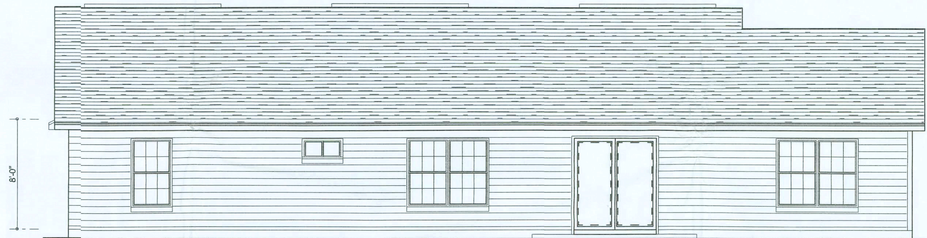
REAR ELEVATION SCALE: 1/4" = 1'-0"
