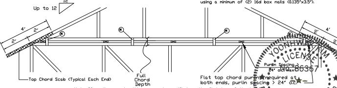
Note: If purlins or sheathing are not specified on the flat top of the back truss, purlins must be installed at 24' o.c. max. and use Detall A. STATE OF
