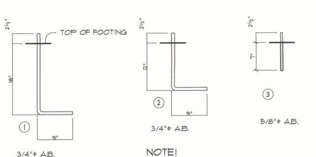
Nr. 3 ANCHOR BOLT SHALL BE SET IN DRILLED 3/4" AX 7" DP. HOLES AND SET WITH 2-PART EPOXY CONSTRUCTION ADHESIVE
